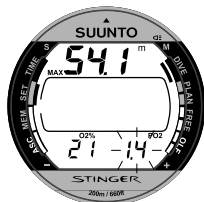
Fig. 4.9. Setting Oxygen Percentage and Partial Pressure.
