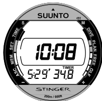
Fig. 2.7. The Stopwatch displays hours, minutes and seconds.
