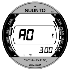
Fig. 4.16. Setting Altitude Adjustment.
