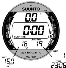
Fig. 3.34. Surface display after Gauge dive. Center window showing surface time.
