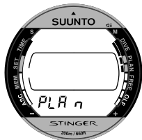
Fig. 3.8. Dive Planning. The Planning mode is indicated by the PLAN text and mode indicators.
