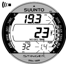
Fig. 3.23. Oxygen partial pressure and OLF displays. There is an audible alarm and the last segment of the bar graph starts to blink as the OLF has reached 80% limit. When OLF has reached 100%, all segments starts to blink. If the OTU value is higher than the CNS value, the lowest segment blinks.
