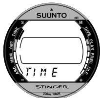
Fig. 2.4. The Time Mode is indicated by the TIME text and a mode indicator.
