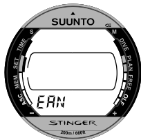
Fig. 4.7. EAN/Air Setting Mode.
