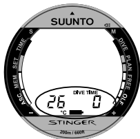
Fig. 3.6. Low Battery Warning. Battery symbol indicates that the battery is low and battery replacement is recommended.
