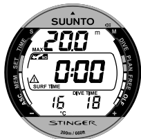
Fig. 3.24. Surface display. You have surfaced from a 18 minute dive, which maximum depth was 20.0 m [66 ft]. The present depth is 0.0 m [0 ft] and surface interval time is 0. Airplane symbol indicates that you should not fly and diver attention symbol indicates that you should prolong your surface interval time because of excess micro-bubbles.
