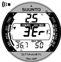
Fig. 3.20. Decompression dive, above ceiling. Note downward pointing arrow, Er warning and an audible alarm. You should immediately (within 3 minutes) descend to or below ceiling.
