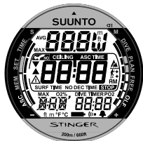
Fig. 3.2. Startup I. All segments shown.
